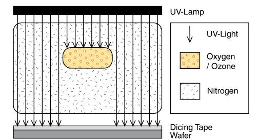
During the UV curing process oxygen  $(O_2)$  is ionized by deep UV light, generating small amounts of ozone  $(O_3)$ . Ozone acts as a filter to the UV light, blocking penetration to the film. That could cause incomplete exposure and adhesive residue on the wafer.
