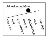
Silicon release agent free uniform thickness medium-high tack adhesive film for direct lamination to the wafer backside. Suitable for use in wafer dicing operations. The base film is of PVC with an acrylic adhesive. Film is supplied in 100-meter rolls without backing liner.
