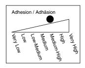
Silicon release agent free smooth medium-high tack adhesive film for direct lamination to the wafer backside. Suitable for use in wafer dicing operations. The base film is of PVC with an acrylic adhesive. Film is supplied in 100-meter rolls without backing liner.
