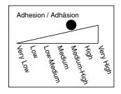
Silicon release agent free, smooth medium tack adhesive for direct lamination to the wafer backside. Suitable for use in wafer dicing operations. The base film is of PVC with an acrylic adhesive. Film is supplied in 100-meter rolls without backing liner.
